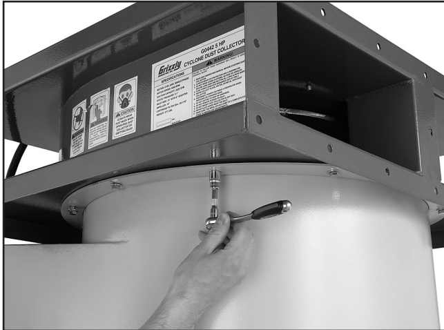
Figure 21. Securing intake barrel assembly to blower housing assembly.
